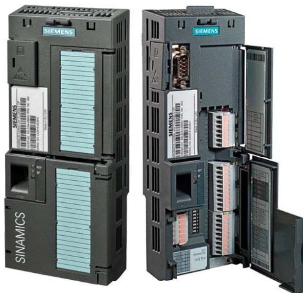
Control Unit CU240B-2 with closed and open terminal covers
