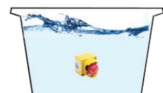
IP67: Submersion to one meter for 30 minutes.
